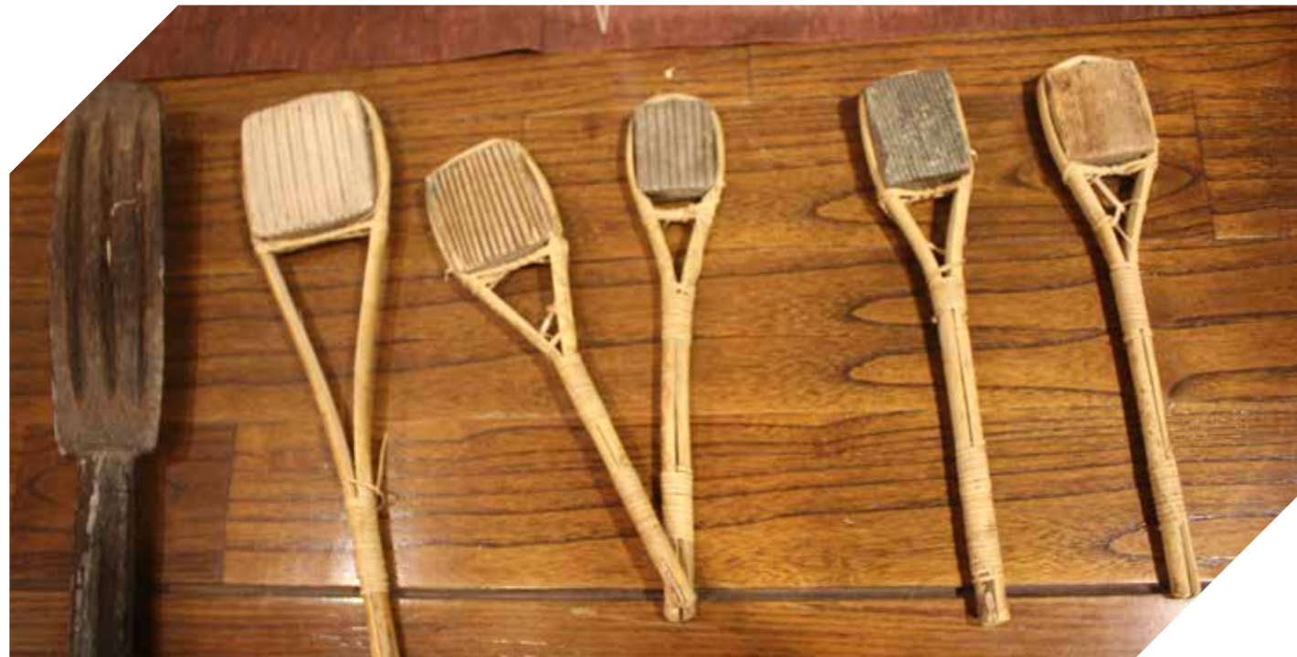
Beating equipment for bark cloth making, made by stone and rattan photo courtesy of Aprina Murwanti Peralatan pukol dalam pembuatan kain kulit kayu, terbuat dari batu dan rotan hak milik foto: Aprina Murwanti
