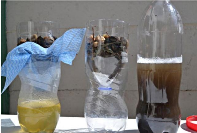
4. As seen in the image, the water is significantly cleaner than when we poured it. You can use the water to water plants or cleaning the floor. Bring out the scientist in you and experiment using different materials and testing as we did in the images below:
