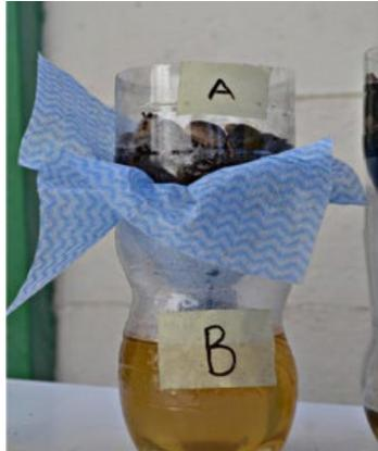
Observation: The water became clearer with the use of Filter A.
