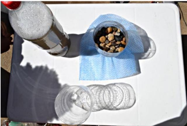
2. Remove the bottle cap and place the cloth over the opening. Secure it with the elastic band. Layer the filtration system using the top part of the bottle, in this order:
