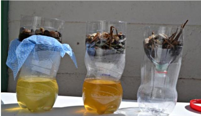
The same greywater was used and the result of the water is evident. Filter A clears better than Filter B.
