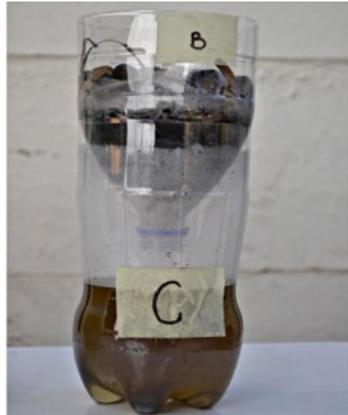
Observation: The charcoal accumulated in Bottle C was almost all filtered out using Filter B.
