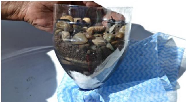
3. Place the filtration system (with the opening facing down) into the bottom part of the bottle and gradually pour the grey/ muddy water. (NB: DO NOT shake the filter).
