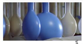
8. Finally, the balloons are inflated with compressed air and pulled off the molds.
