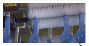
5. One makes the rolled edge with a brush.
