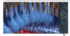
6. The molds are then put in the oven.
